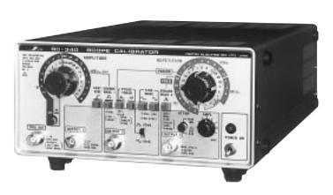
0.12 mV - 60 V 0.2 mV - 100 V 0.1 ms - 2 s 0.5 Hz - 1 MHz The SC-340 is a signal generator for checking and calibrating the deflection factor, sweep rate, pulse response, and triggering of oscilloscopes with bandwidths up to 100 MHz.
