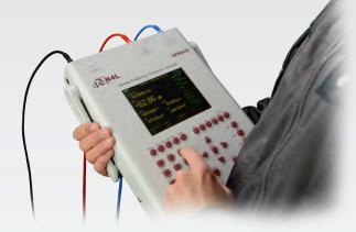
Set up the sweep and enter transformer parameters, save sweep to the SFRA45's 1GB internal memory
